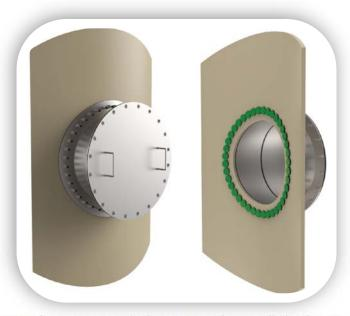
The remarkable performance track record of our fittings and side manways is testament to the importance of stress elimination on both the tank and the fitting. Available in fiberglass and stainless steel as standard. Hardware options include 316SS, titanium, and C-276 Hastelloy. Standard gaskets options are EPDM and Viton. We have been granted U.S. Patent no. 9,464,745 for our fiberglass version of large fittings including side manways.
